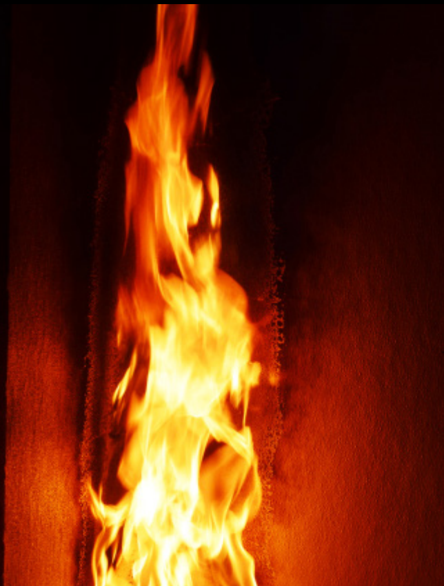
Fire development test (SBI - Single Burning Item Test)
